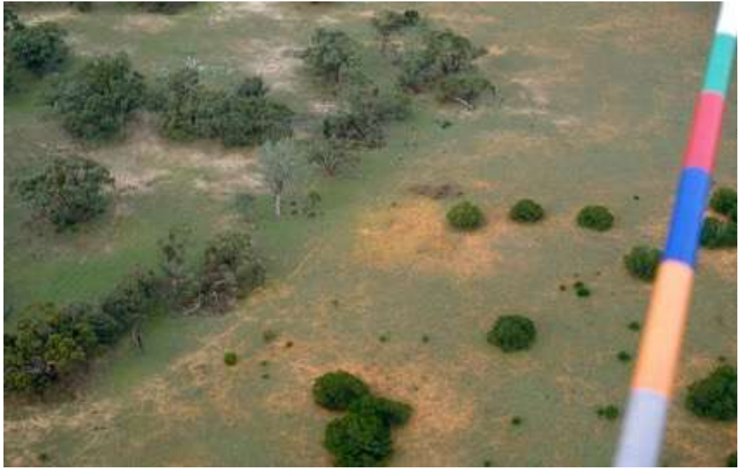
Figure 31. Part of an observer's view of the ground from the open side of a helicopter fitted with a colour-banded horizontal sighting rod. Animals on the ground are recorded in their original positions as the rod sweeps over them, and recorded in the form: 'blue: 4', 'green: 1', 'grey: 2', 'blue: 1', and so on. Animals that take fright and have started to run when the observer first detects them present a problem ( see text ).
