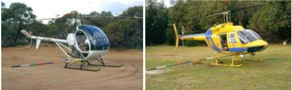
Figure 30. A sighting rod fitted to two small helicopters, the 'Hughes 300' ( left ) and to a medium-sized helicopter, a 'Bell Jet Ranger' ( right ). The rod is colour-banded in strips of different colours but equal width. The observer sits, with shoulder-belts attached, and leans slightly out of the aircraft so that it is possible to look directly down as well as to the side. Notice that, in many countries, attachment of a sighting rod is considered an engineering modification that also requires flight-testing before its use can be approved.
