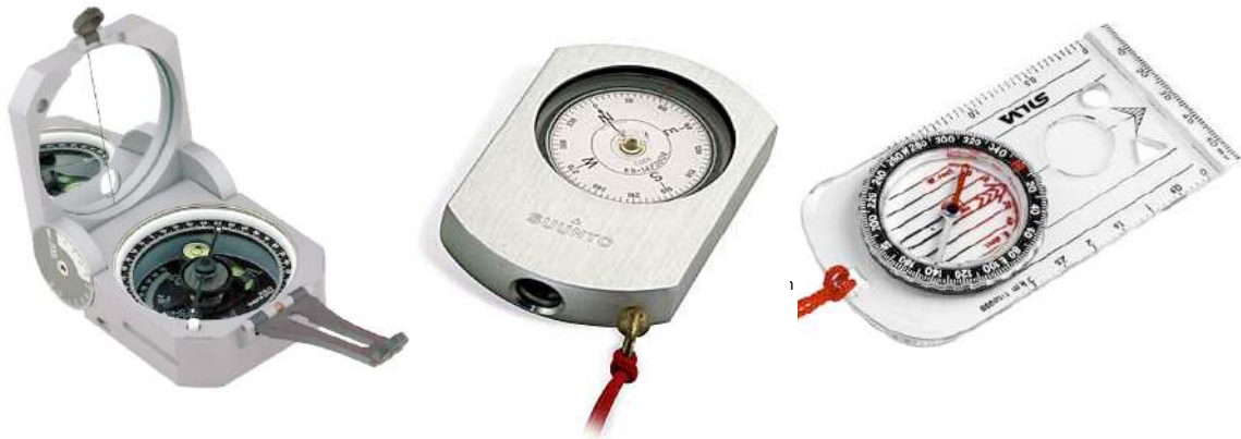
Figure 14. Three types of magnetic compass: a 'Brunton Transit' lensatic compass (left), a 'Suunto RD' compass (centre), and a 'Silva NL Explorer' orienteeing compass (right). All three are suitable for line transect work, but vary in capabilities and price. The 'Silva' orienteeing compass shown is cheapest, easy-to-use, fine for navigation when used correctly, and just adequate for measuring bearings to detection points if these are needed. The 'Suunto' model shown costs more, is more accurate, easier to use for taking bearings, but a little less convenient for navigation. The 'Brunton' model shown is most accurate, best for navigation and best for taking bearings, but also the most expensive. If you are on a budget and are relying on detection distances from the observer as your technique, then an orienteeing compass is 'best buy'.
